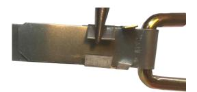
6. Using a pair of pliers fold the rear lugs down tight on the strap. (See figure above.)
